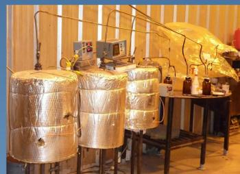
Insulated and Assembled Soak Test Units
